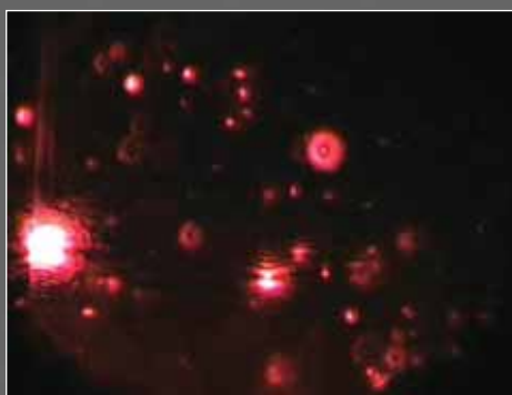
Analysis image of a clearly polydisperse material, showing the wide range of scattering intensities (Titanium Dioxide in water).
