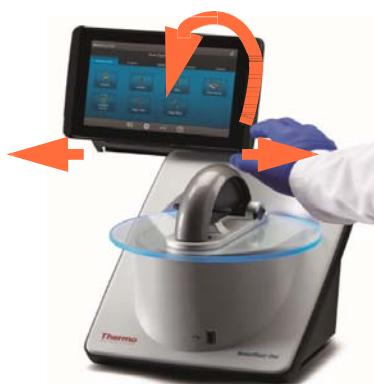
Load blank or sample and close the arm quickly to initiate measurement
